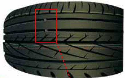
TWI (Tread Wear Indicator) – with the limit value of 1.6mm.
